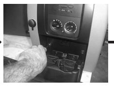
**STEP 12:** With the console out of the Expedition, pull down the rear cup holders. Us e a 7mm bolts that have been exposed.
